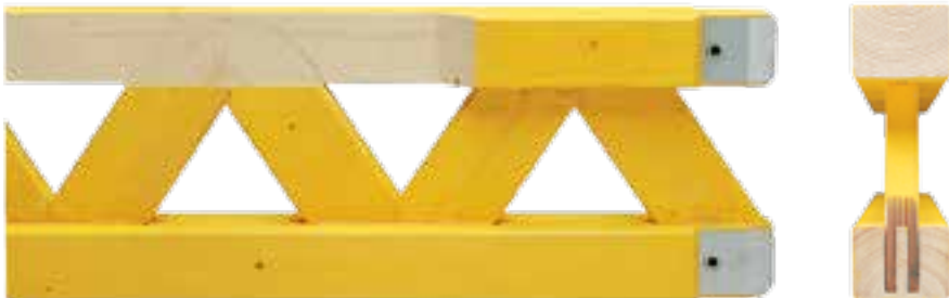
The girder nodes with mini-dovetail jointing guarantee the durability of the GT 24 Lattice Girder. The struts penetrate the chords along the whole cross-section and there are practically no cavities which could collect and hold moisture.
